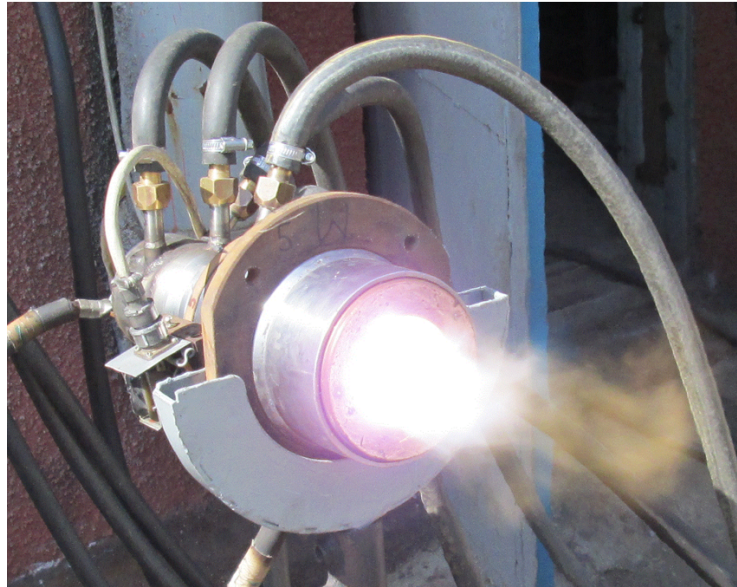
Figure 3. VORTEX-200 linear circuit electric arc plasmatron during the test.
