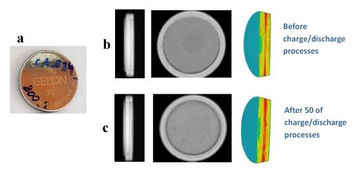
Figure 3. a) The photograph of a lithium-ion battery, b) radiographic images and a slice of a 3D model at the initial stage, and c) radiographic images and a slice of a 3D model after 50 charge-recharge cycles.
