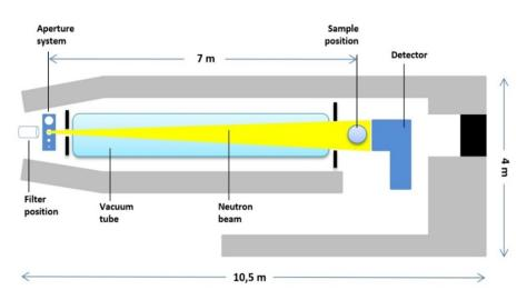
Figure 1. The layout of TITAN neutron imaging facility at the WWR-K reactor.
