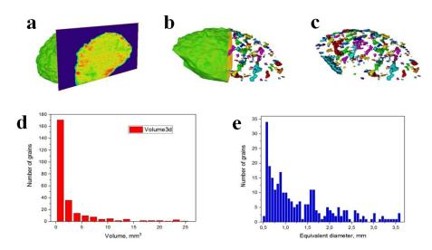
Figure 5. a) An example of a slice cut of the three dimensional model; b-c) 3D model of separated grains of pyrite mineral after segmentation processes. Colours correspond to different grain sizes; d-e) Distribution of grains of the pyrite by volume and equivalent diameter.
