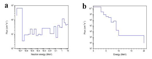
Figure 2. The spectra of (a) neutron and (b) gamma radiation simulated using the MCNP program for channel No. 1 of the WWR-K reactor.
