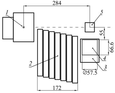
Figure 2. The experimental setup with HPGe: 1 - ING-27 neutron generator; 2 - lead shield; 3 - HPGe  $~\gamma$  -detector; 4 - sample.
