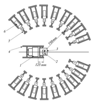
Figure 1. The experimental setup "Romasha": 1 - ING-27 neutron generator; 2 - target; 3 - target holder; 4 - aluminum frame of the setup; 5 - supports for  $\gamma$  -radiation detectors; 6 -  $\gamma$  -radiation detectors; numbered from 1 to 18.
