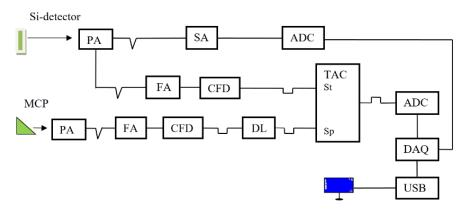
Figure 10. Block scheme of electronics when using a signal from the MCP and Si-detector.
