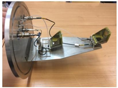
Figure 5. General view of the time-of-flight spectrometer.
