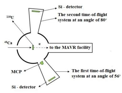
Figure 9. Diagram of a two-arm time-of-flight spectrometer consisting of a reaction chamber and time-of-flight arms based on MCP detectors and Si detectors with an area of  $55 \times 55$  mm<sup>2</sup>.
