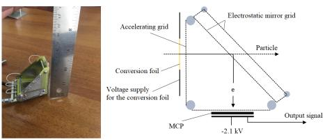
Figure 1. The scheme of MCP detector.
