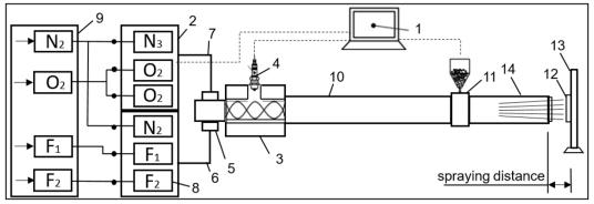
Figure 1. Schematic diagram of CCDS2000 detonation system: 1-control computer, 2-gas distributor, 3-mixing-ignition chamber, 4-spark plug, 5-barrel valve, 6-fuel line, 7-oxygen line, 8-gas valves, 9-gas supply unit, 10-breech block, 11-powder batcher, 12-workpiece, 13-manipulator, 14-muzzle of the barrel.
