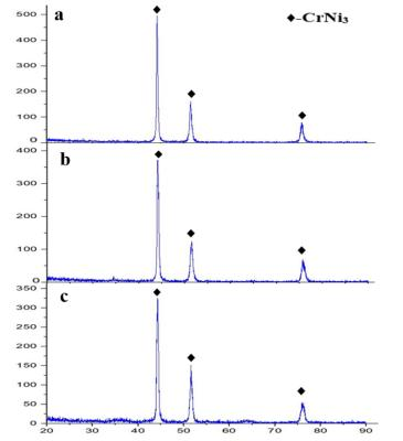
Figure 3. Diffractograms of the NiCr coatings received at filling 58% (a), 54% (b), 65% (c).
