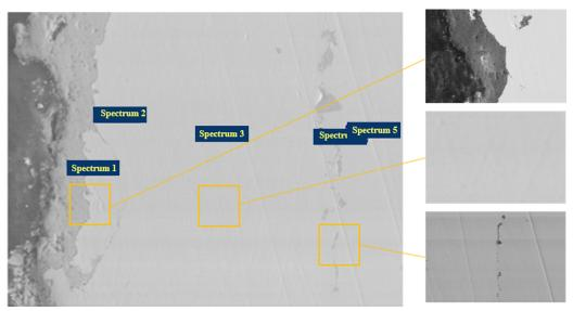
Figure 4. SEM cross-sectional image of multilayer coating on the bases of NiCr/NiCr  $Al_2O_3$  /  $Al_2O_3$ .
