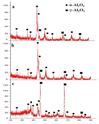
Figure 2. Diffractograms of  $Al_2O_3$  coatings obtained at barrel filling volume 63% (a), 54% (b), 45% (c).
