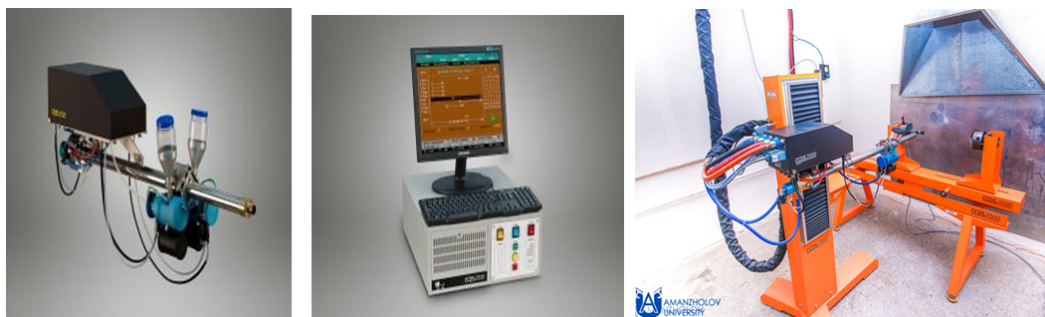
Figure 2. Detonation complex CCDS2000: a) working body (gun) consisting of a barrel, a gas distribution unit and powder dispensers; b) the control unit on the basis of the industrial computer; c) the gun is complete with a 3-coordinate manipulator.
