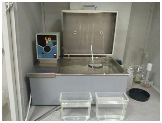
Figure 1. The device of a water bath for chemical etching of film samples.
