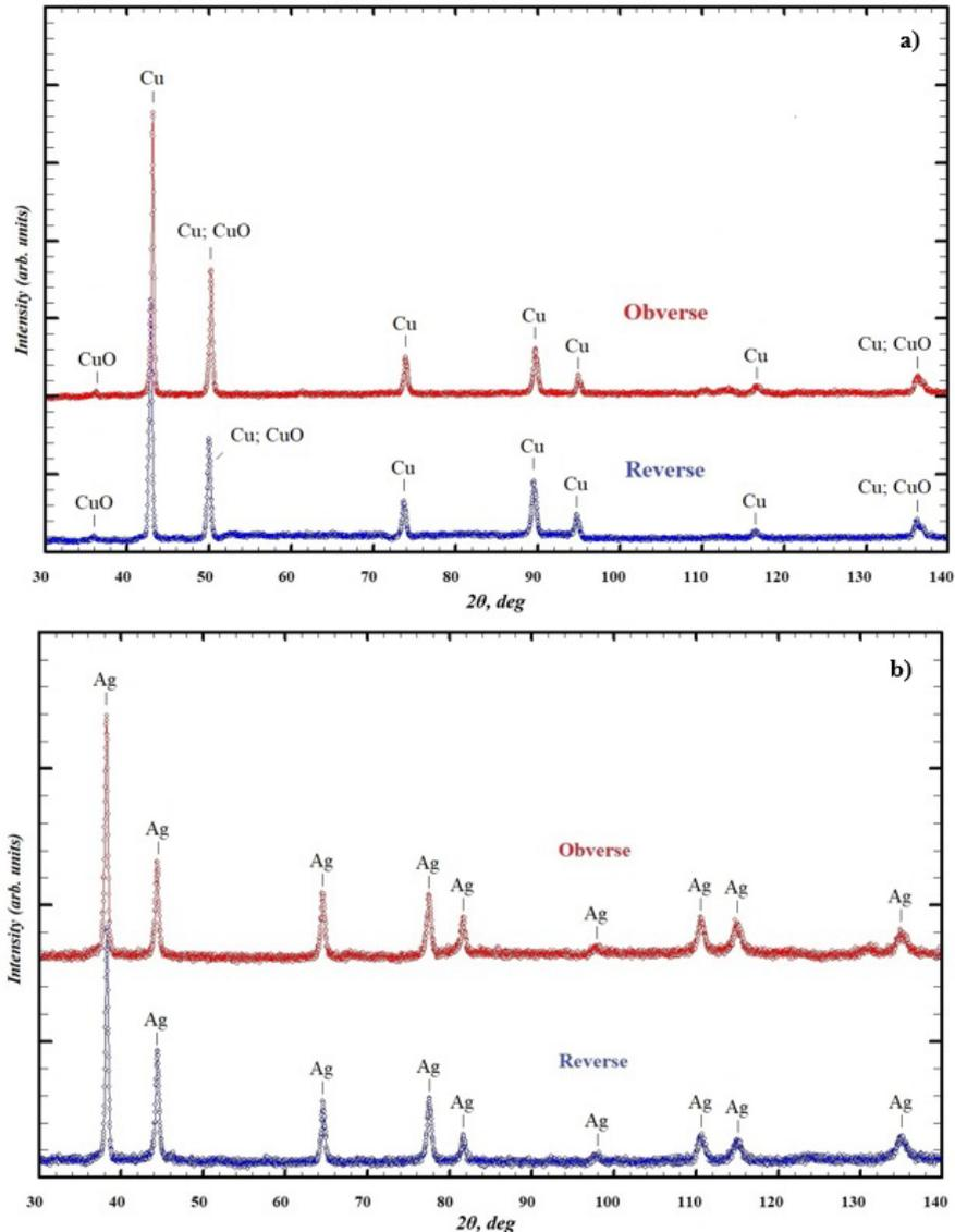
Figure 2. X-ray diffraction spectra of the obverse and reverse sides of the copper coin of Heliocles (a) and the silver coin of Demetrius (b). The figure shows the experimental data and the calculated profile obtained by the Rietveld method. The diffraction peaks in the obtained results correspond to the phases of copper, silver and tenorite. The Miller indices for cubic phases of copper and silver are indicated.
