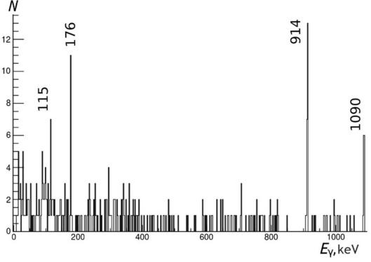
Figure 1. Spectrum of detected  $\gamma$  -quants from the decay of <sup>250</sup> No.  $E_{\gamma}$  -  $\gamma$  -quants energy. N -counts.
