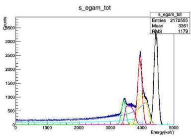
Figure 1. Model response function and its components.
