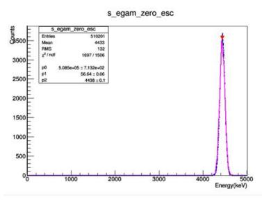
Figure 2. Peak of total absorption.
