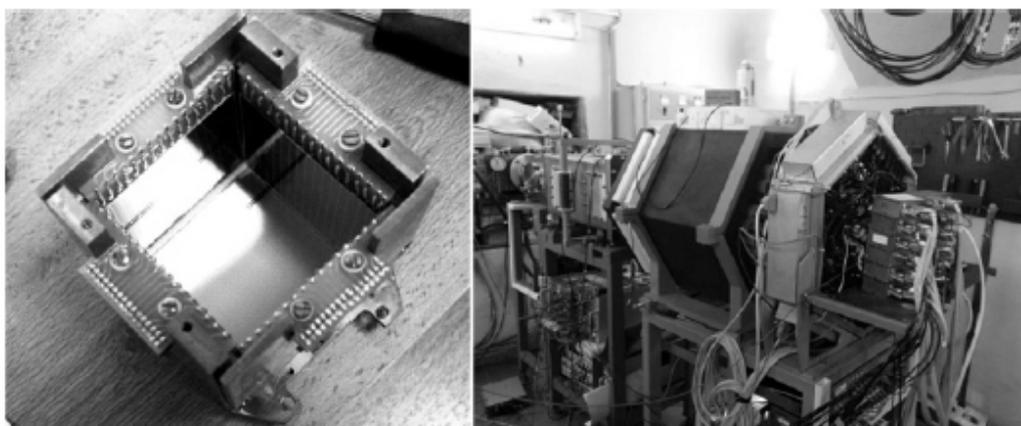
Figure 2. Array of silicon strip detectors (left) and neutron detector (right).
