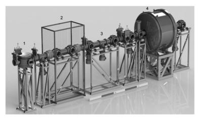
Figure 4. Model of the measuring facility with a Penning ion-trap (4). (1) is a turning magnet, (2) indicates the gas-filled RFQ, (3) is the multi-ToF system.
