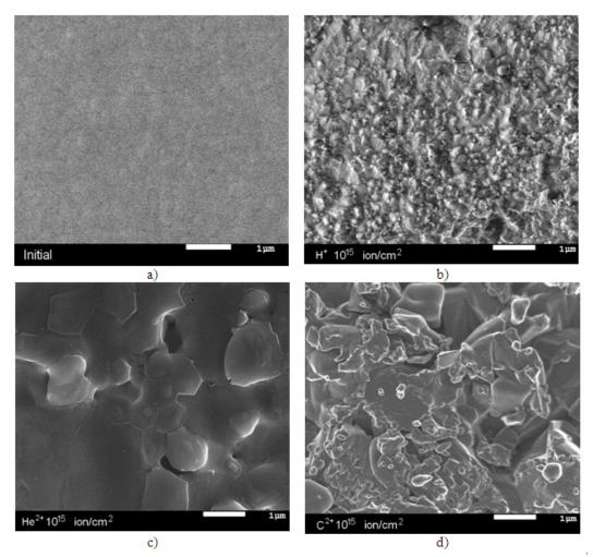
Figure 2. SEM images of the studied ceramics before and after irradiation: a) Initial; b) H + 10<sup>15</sup> ion/cm<sup>2</sup>; c) He<sup> $^{1}$ </sup> + 10<sup>15</sup> ion/cm<sup>2</sup>; c) He<sup> $^{1}$ </sup> + 10<sup>15</sup> ion/cm<sup>2</sup>; c) He<sup> $^{1}$ </sup>
