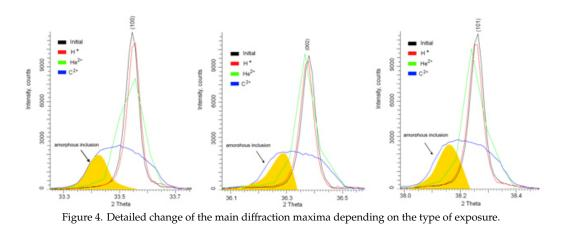
As can be seen from the presented data (Figure 3-4) for the samples irradiated with protons, the change in diffraction peaks, which reflects the change in stress concentration and deformations in the structure, is insignificant. Moreover, there is no significant shift in the diffraction maxima. This indicates a low concentration
