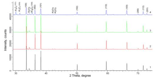
Figure 3. X-ray diffraction patterns of the studied ceramics before and after irradiation: 1) initial; 2) proton irradiation; 3) irradiation with He<sup>2+</sup> ions; 4) irradiation with C<sup>2+</sup> ions.
