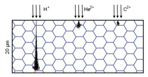
Figure 1. Schematic representation of the trajectory of the passage of ions in ceramics.
